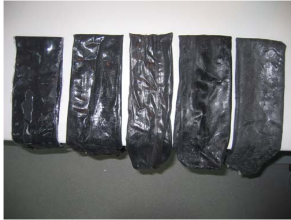
Figure 16 - Licra fibre in silicone matrix composite material for the wing skin
